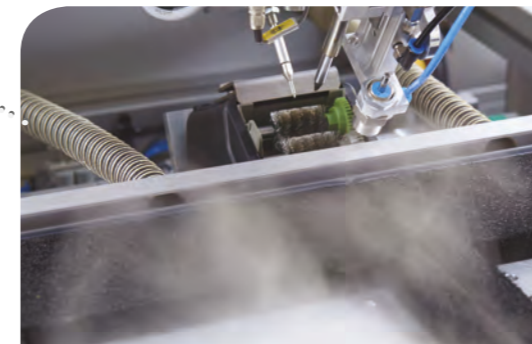
Safety cover fully encloses the integrated fume extraction system, protecting the user, workpiece, and equipment
