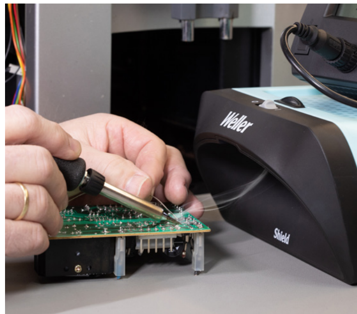
Soldering with fume extraction
